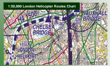
This chart is for the purpose of visual air navigation for helicopters within the London area, and can be also used in preflight planning and for pilot and navigator training. It depicts the current helicopter routes into and out of the London area, Heliports, Altitude Limits and reporting points.
